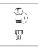
1. Connect the supply pipe by screwing it to a cold water tab using a <sup>3</sup>/<sub>4</sub> gas threaded connection (see *figure*). Before performing the connection, allow the water to run freely until it is perfectly clear.
